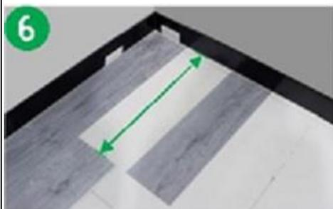
Any offcuts with minimum of 30cm can be used to start the new row which ensures a natural random joint structure.
